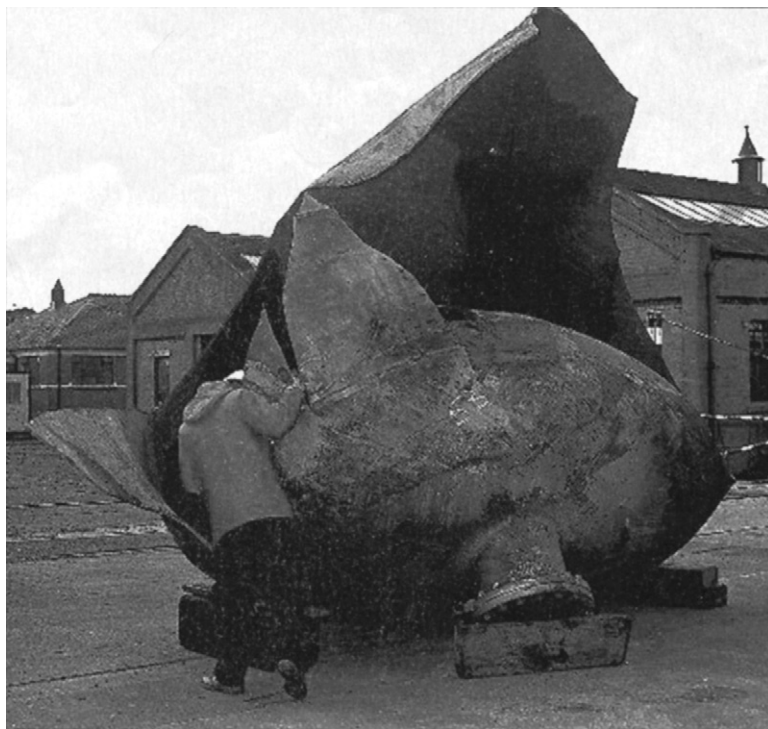
FIGURE 28-1 The result of an absorber failure. From reference 18. (Reprinted with the permission of Gulf Professional Publishing.)
