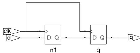
Figure 4.18 sync synthesized circuit
