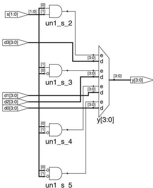
**Figure 4.7** mux4 synthesized circuit
