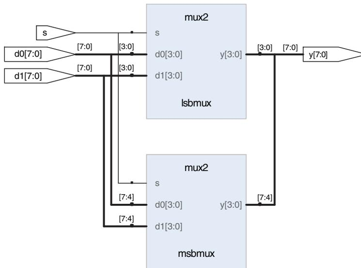
**Figure 4.13** mux2\_8 synthesized circuit
