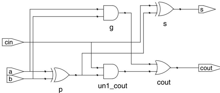
**Figure 4.8** fulladder synthesized circuit
