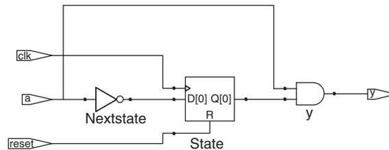
**Figure 4.27** patternMealy synthesized circuit**4.7 DATA TYPES\***
