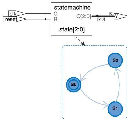
**Figure 4.25** divideby3fsm synthesized circuit
